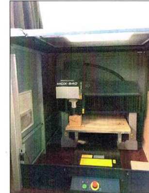
Then I put it onto the wood miller to cut the mould.
